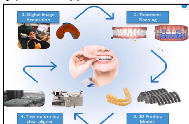
Fig 6 : Workflow of fabrication of clear aligners by the thermoforming process.
